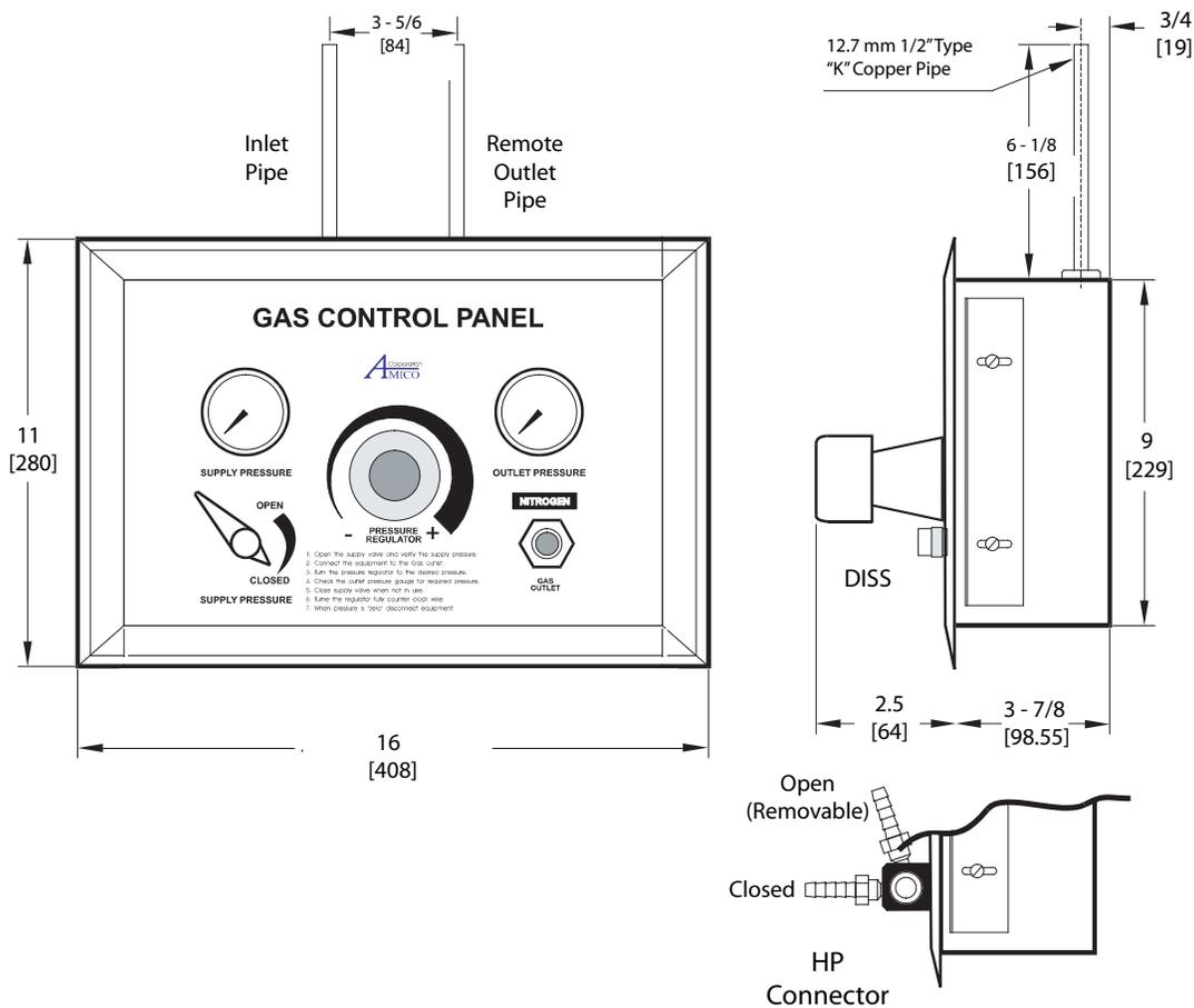
**N-X-CON-ADA-B25** = High pressure adapter with 1/4" Hose barb. (supplied with HP Gas Control Panel).
